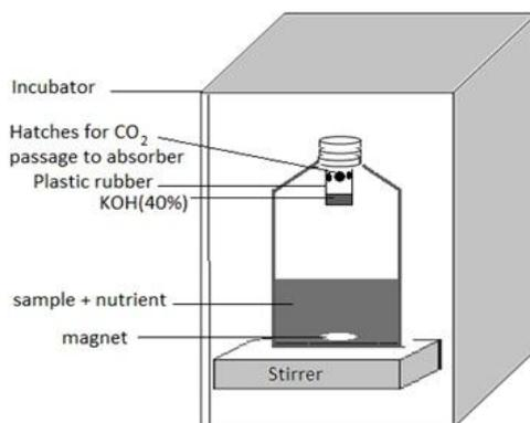
Figure 1: Schematic apparatus used for BOD measurement.
